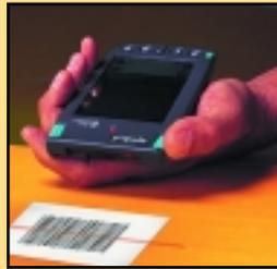
Designed by Symbol Technologies and Palm Inc., the SPT 1500 combines bar code scanning technology with Palm OS platform.
